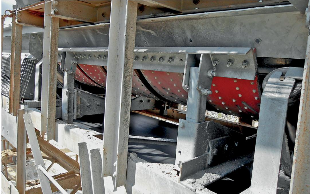
The patented **FLEXAL**® system provides an ideal solution to the problem of punching on the belt in reception areas.
